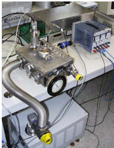
Fig. 7: Test setup with RIVA sensor mounted on the vacuum vessel in center, HV switch in background
