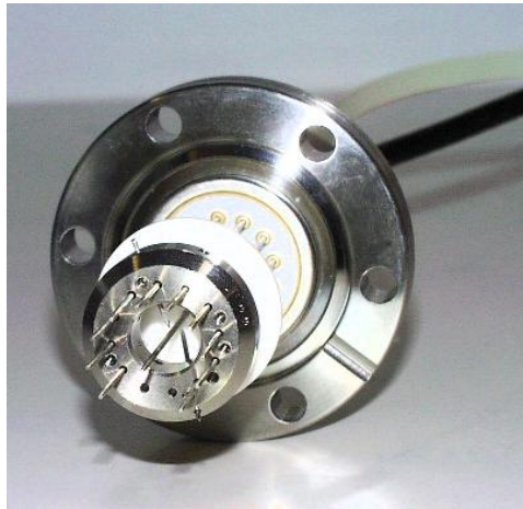
Fig. 6: Needle anodes placed in different distances to a cylindric kathode.
