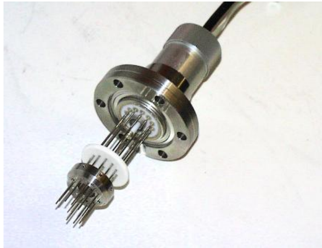
Fig. 2: The RIVA sensor with plug and analog electronics
