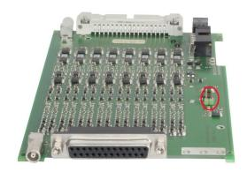
On the right side the power select jumper can be seen. When open, high power is selected (default at delivery).
